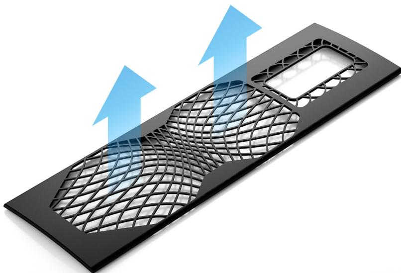
*Even the layout of the grille pattern was subject to serious experimenting. There are no similar sized holes, the benefit being that the cloth stays silent on the grille itself. Multiple, identical holes would cause the cloth to vibrate on the grille as the airflow through each hole would be identical.*
