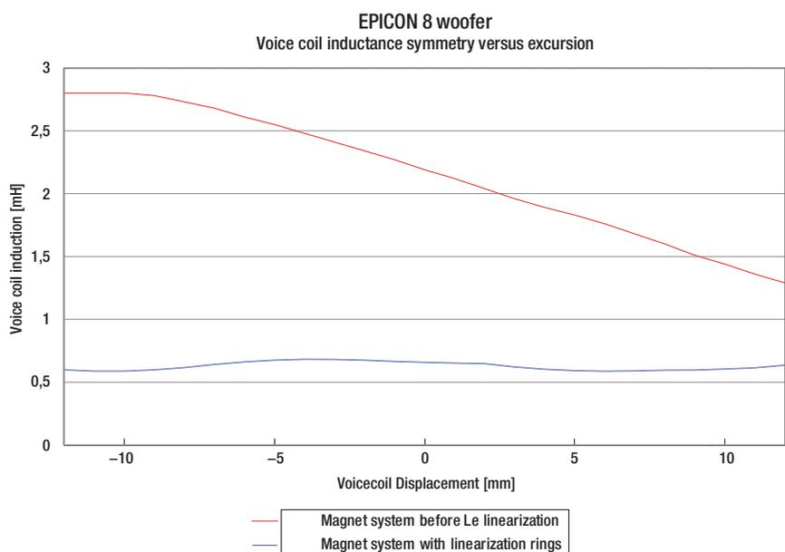
Voice coil inductance as a function of excursion is shown on the lower curve, compared to an identical design, only without linearization rings (the upper curves).
