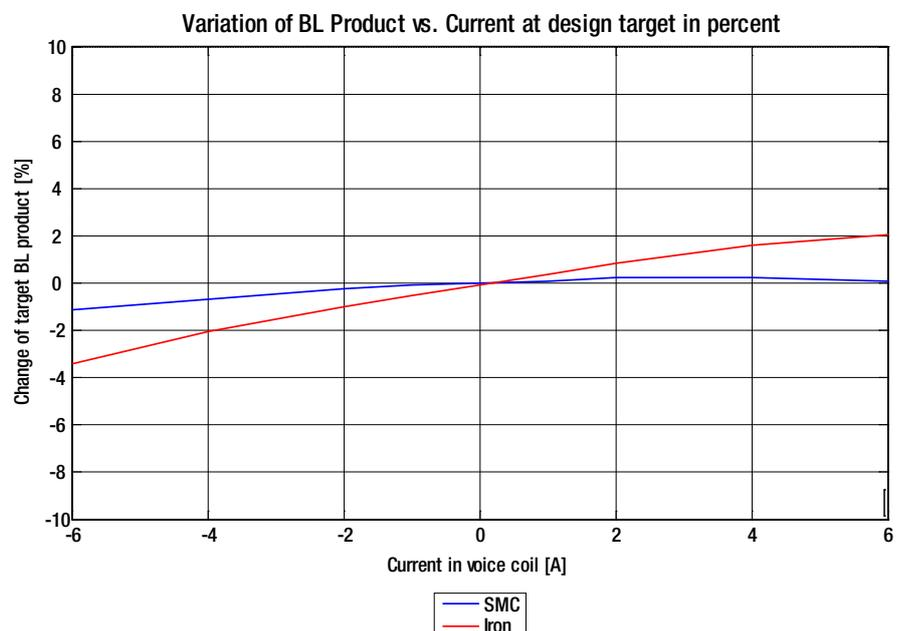
However, a real substantial reduction of the current-generated flux modulation, can be only obtained by using electrically non-conductive materials near the magnet gap, - as this part of the magnet system is (by nature of a magnet system design) very close to the voice coil.
