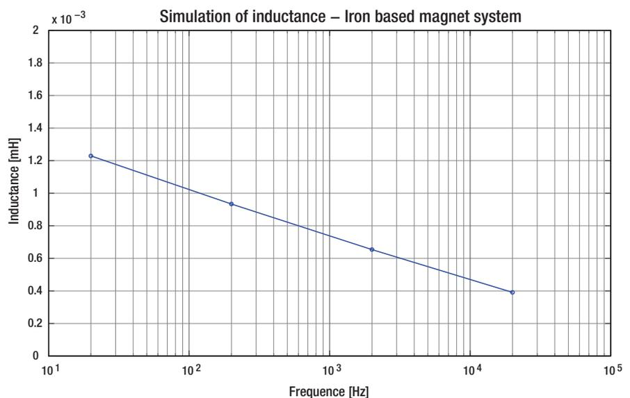
Furthermore, the SMC material offers very frequency linear magnetic properties. This means that the voice coil inductance - and thus the conversion of the amplifier voltage
