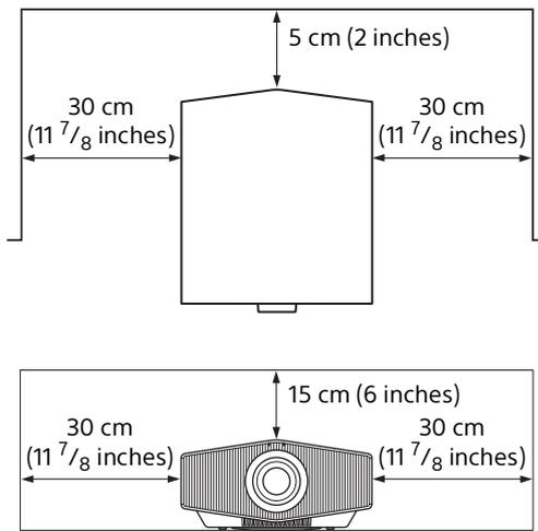
Note that the wall on the ventilation holes side may become hot. Air from air conditioners or the ventilation holes of this unit or other devices, may cause oscillation on the screen. Be sure not to install this unit in the area where the air from air conditioners or the ventilation holes of these devices reach to the front side of this unit.
