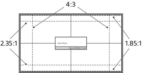
The dashed lines show the angle of view of each aspect ratio.
