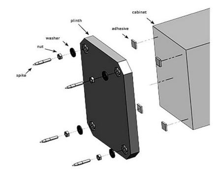
Thread a nut onto the spike. Next, slide a silicone washer into the spike assembly. Insert the assembly into the plinths. Repeat this procedure until all 8 spikes are fastened into the plinths. Once all the spikes and washers are installed level the plinth to the floor.
