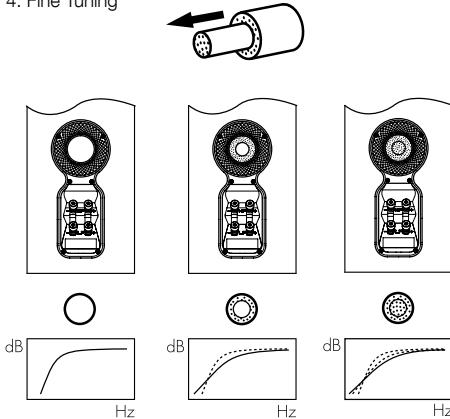
Before fine tuning, make sure that all the connections in the installation are correct and secure.
