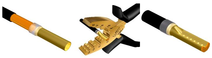
Wire is stripped and the appropriate size crimp sleeve is slid onto the strands.
